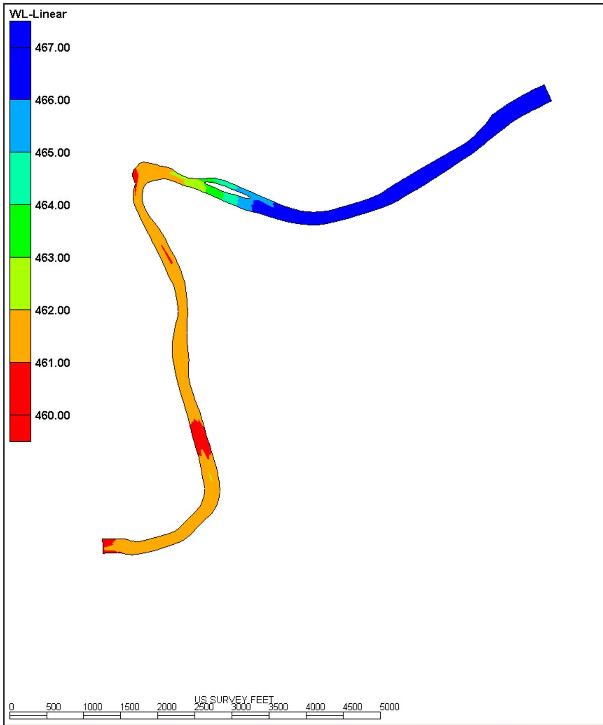
Figure 12: Interpolation of water surface survey data onto model grid
