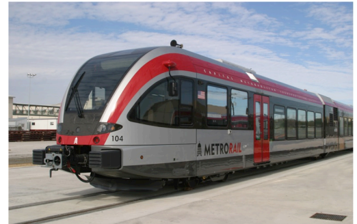
Made by Stadler, the rail vehicle above is an FRA Alternatively Compliant train.
