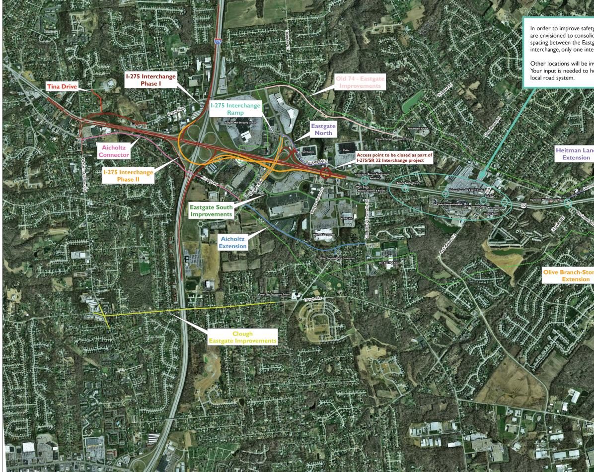
In order to improve safety and reduce congestion, the SR 32 Eastgate Area Improvements are envisioned to consolidate and manage access points along SR 32. Based upon required spacing between the Eastgate Boulevard Interchange and the Olive Branch-Stonelick Road interchange, only one interchange can be provided, somewhere within this area.
