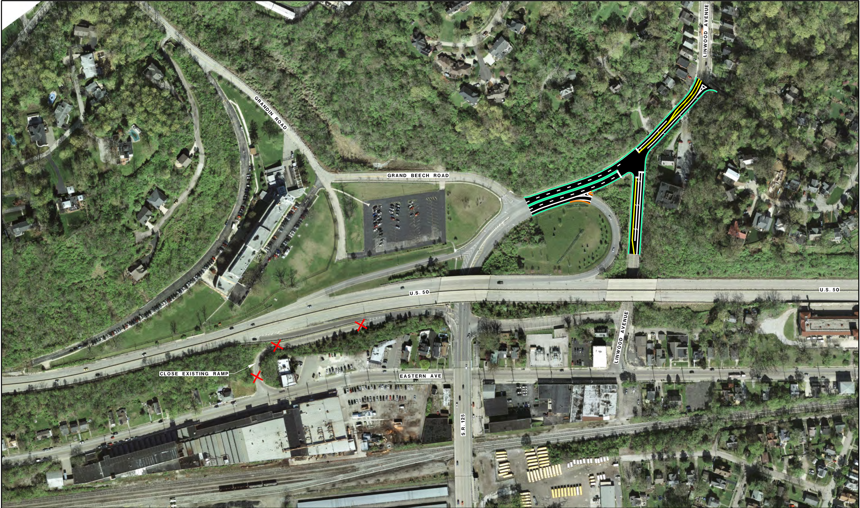
Figure I-29B & X-3B CLOSURE OF GEOMETRICALLY DEFICIENT RAMP FROM EASTERN AVE TO S.R. 125 AND REPLACEMENT WITH INTERSECTION AT LINWOOD AVENUE
