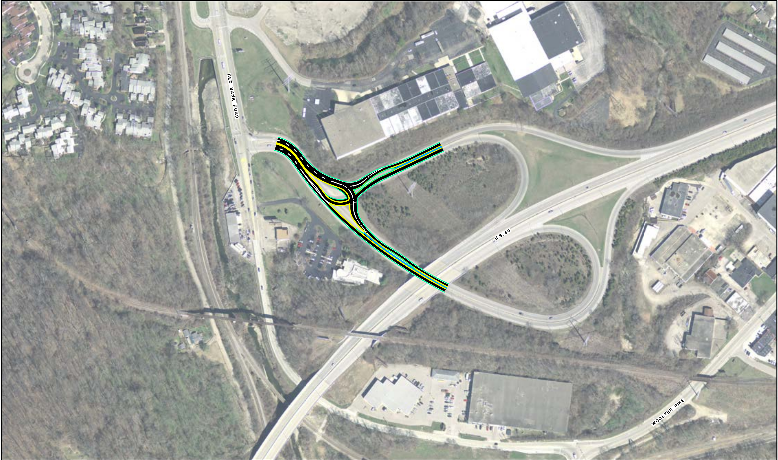
Figure X-4C-2 ROUNDBOUT AT COLBANK AND U.S. 50 RAMP INTERSECTION
