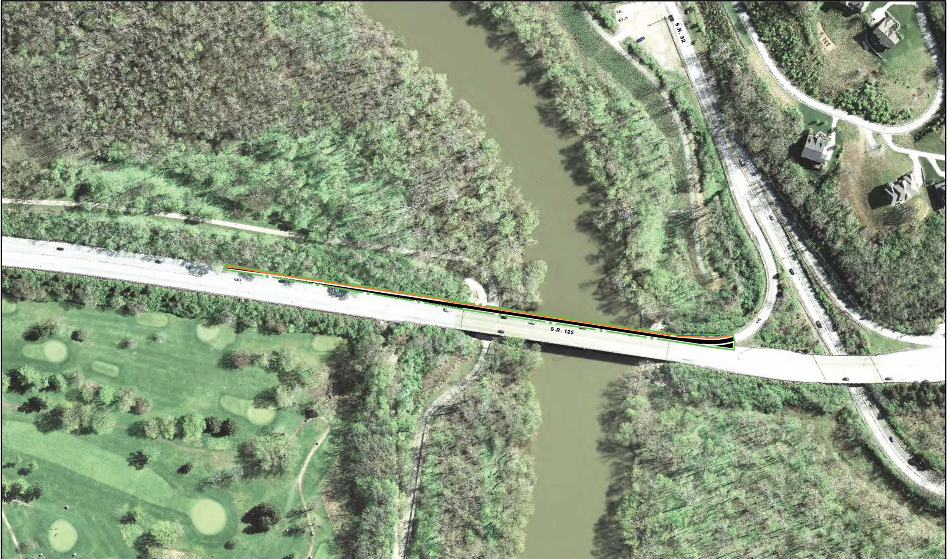
Figure X-1C EXTEND MERGE LENGTH ON RAMP FROM WESTBOUND S.R. 32 TO WESTBOUND S.R. 125
