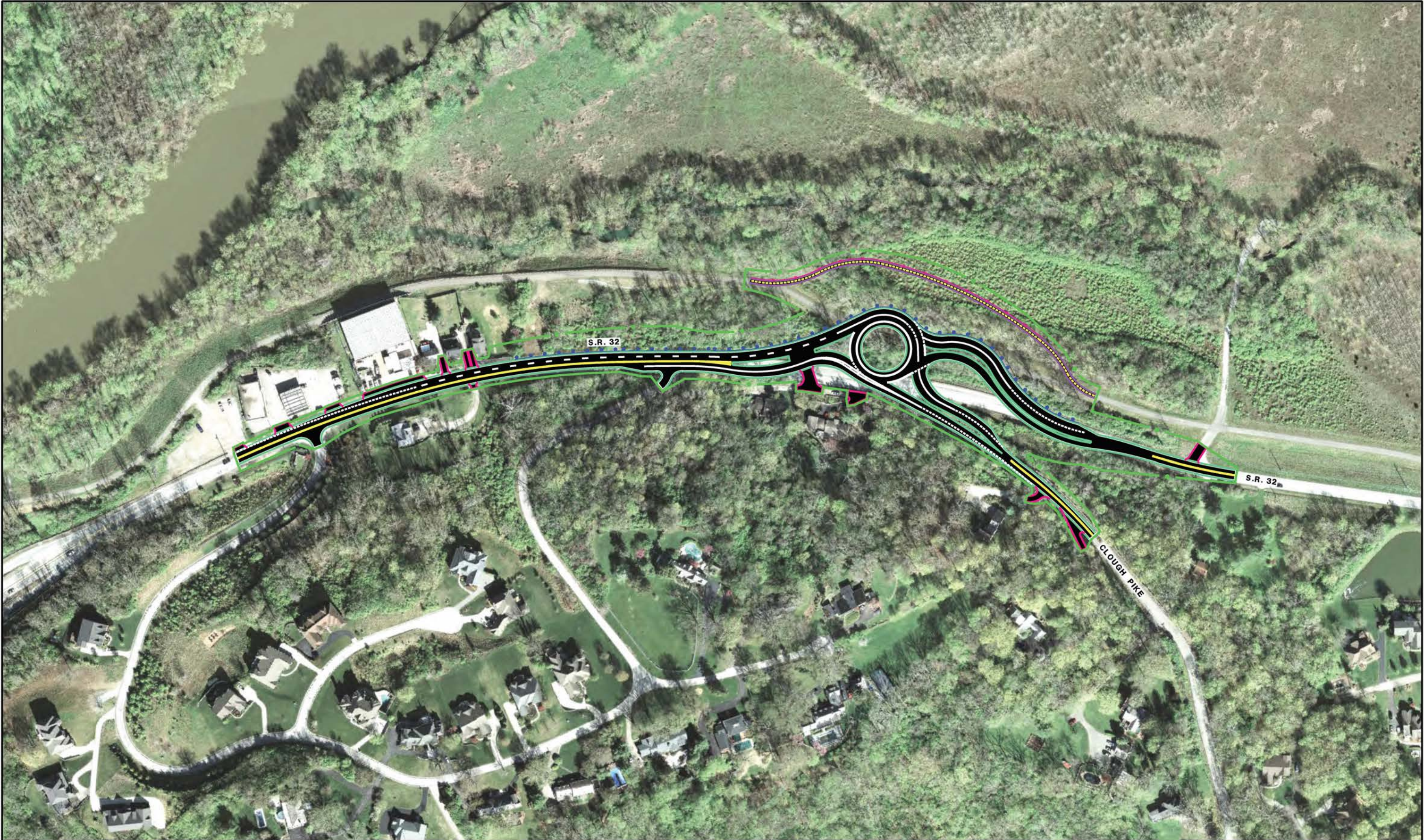
Figure I-7C ROUNDBOUT AT S.R. 32 AND CLOUGH PIKE INTERSECTION AND RELOCATED BIKE TRAIL
