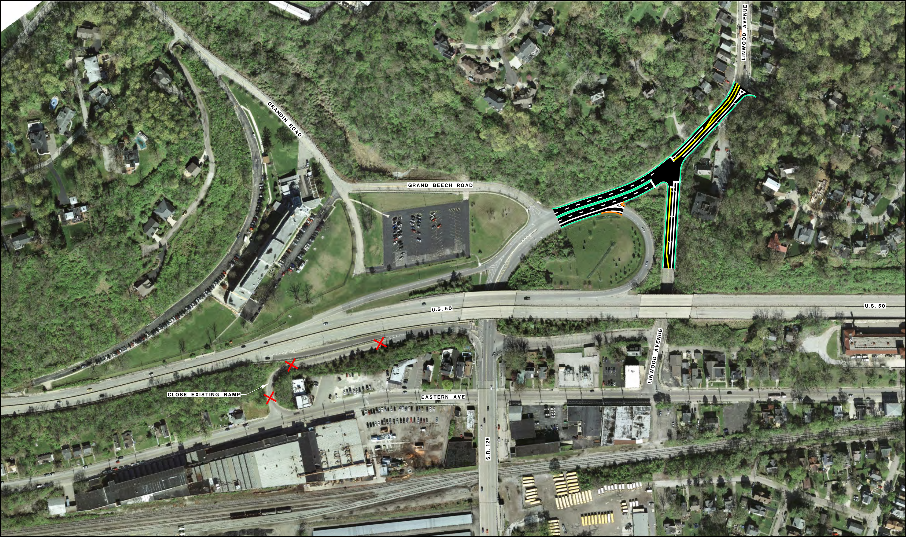
Figure I-29B & X-3B CLOSURE OF GEOMETRICALLY DEFICIENT RAMP FROM EASTERN AVE TO S.R. 125 AND REPLACEMENT WITH INTERSECTION AT LINWOOD AVENUE
