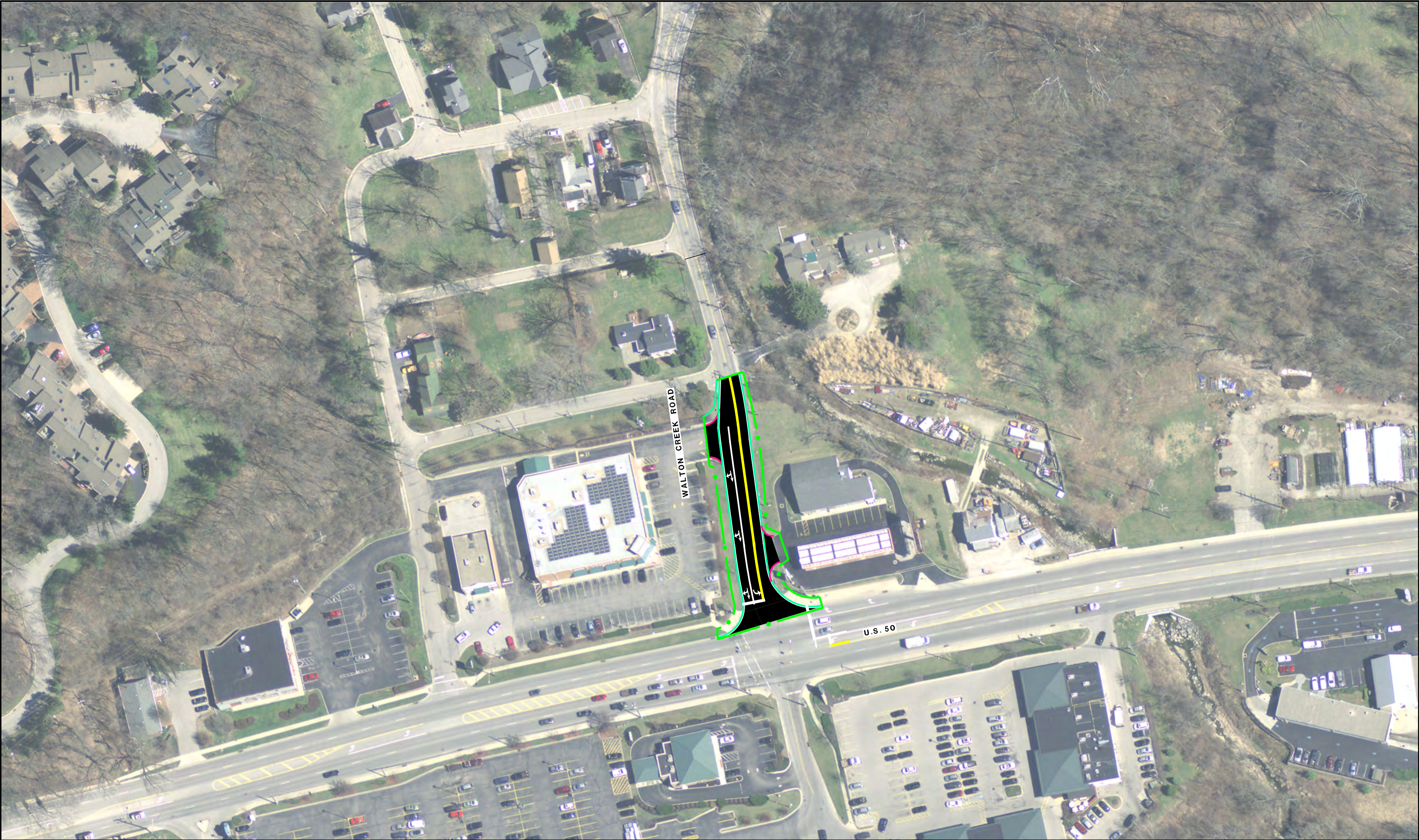
Figure I-12B ADD PROTECTED/PERMISSIVE SB LEFT TURN PHASE AT WALTON CREEK/ US 50 INTERSECTION
